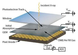
Fig. 2. Schematic of the polarization-sensitive gas pixel detector.
